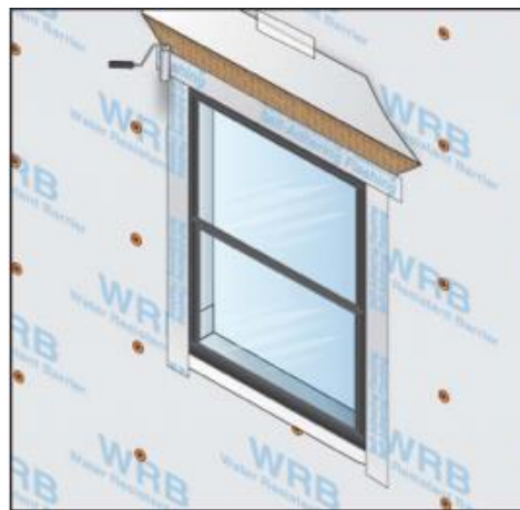
Figure 9. Flashing installation method (FMA/AAMA 100-12 2012)
